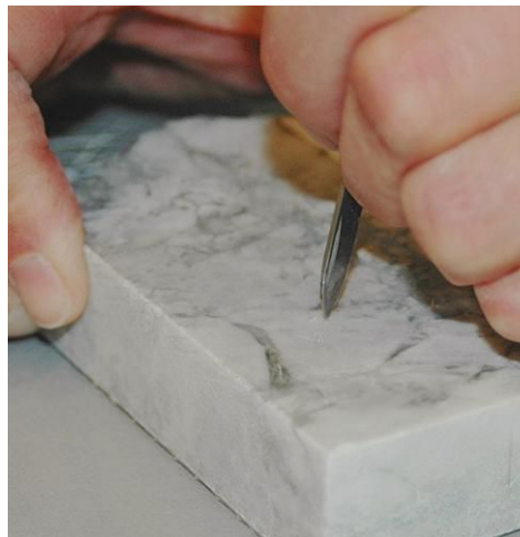
The knife blade test. Photo © Karin Kirk
