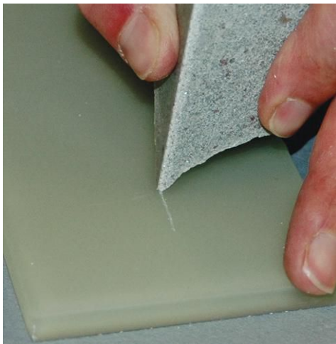
The glass scratch test. Photo © Karin Kirk
